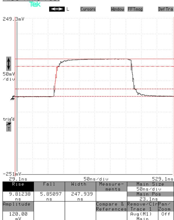
Output of AVX-MRB6 into 3.1Ω, in response to a 500 mV pulse with ~300 ps rise time.
