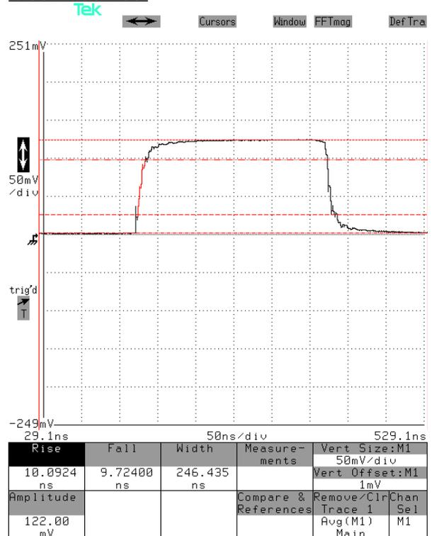
Output of AVX-MRB6 into 3.1Ω, in response to a 500 mV pulse with ~300 ps rise time.
