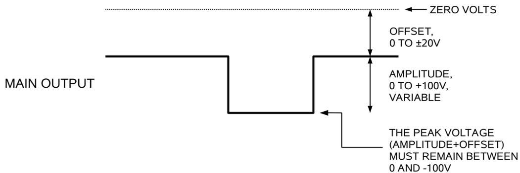
⚠ If the user adjusts offset and amplitude values from the front panel, it is possible to get into a condition where a DC offset value is set, which then prohibits an amplitude from being adjusted on the rotary dial. For example, if the DC offset is set to -20V, and the user then tries to increase the amplitude from its default setting of 0V, an error will occur, because the next step above zero (+100mV) would violate the rules (it needs to be > +20V).
