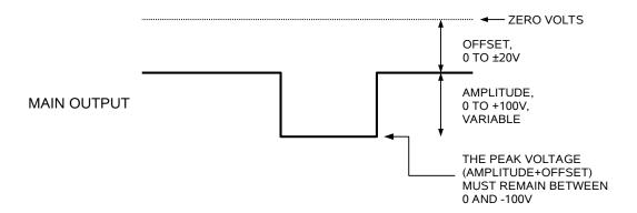
$\bigcirc$  If the user adjusts offset and amplitude values from the front panel, it is possible to get into a condition where a DC offset value is set, which then prohibits an amplitude from being adjusted on the rotary dial. For example, if the DC offset is set to -20V, and the user then tries to increase the amplitude from its default setting of 0V, an error will occur, because the next step above zero (+100mV) would violate the rules (it needs to be > +20V).
