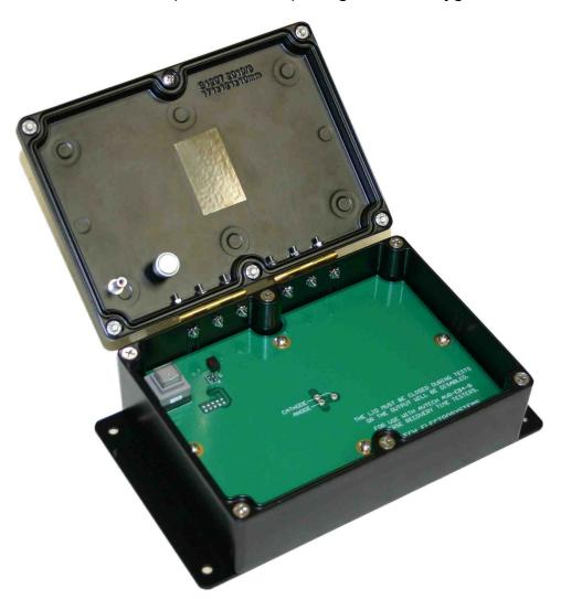
The AVX-TRR-TO254AA accepts TO-254AA packages. The test jig is shown below:
