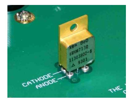
The next photo below shows a TO-254AA package installed so that pin 1 (on the left) is used as the anode, and pin 2 (in the middle) is the cathode. Pin 3 (on the right) is unused:
