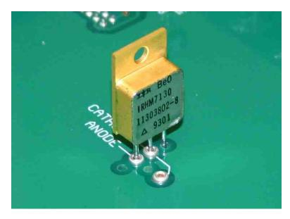
By rotating the package appropriately, all possible pin configurations can be accommodated.
