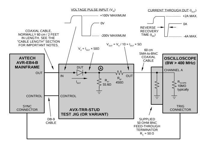
$\triangle$  A 50 Ohm resistance (R<sub>c</sub> in the diagram above) must be connected to ground on the output. This can be a discrete resistor, a feed-through terminator, or the input impedance of an oscilloscope. If a high-speed sampling oscilloscope is used, the input should be protected by adding attenuator on the input. In the diagram above, the 50 Ohm feed-through terminator supplied with the AVR-EB4-B is used to provide the required 50 Ohm resistance.
