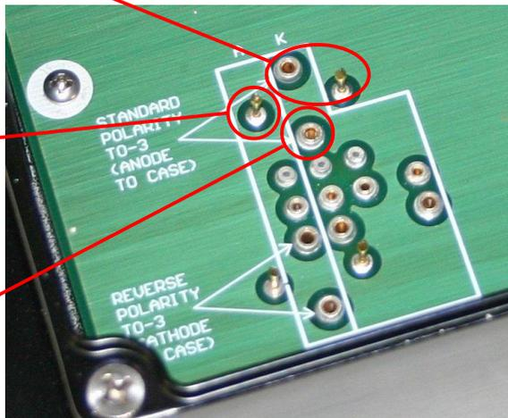
If the case is connected to the cathode, and the pin(s) are used for the anode, the arrangement shown below must be used:
