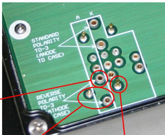
This spring pin must contact the underside of the case. It provides the cathode connection.
