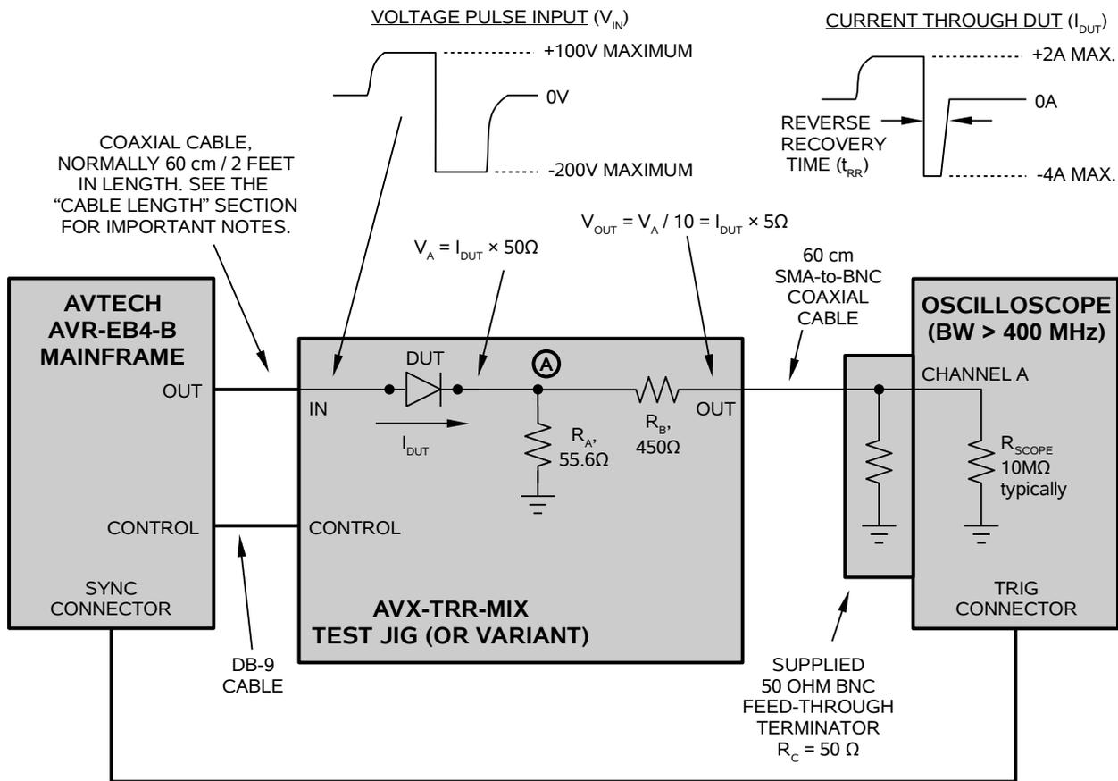
⚠ A 50 Ohm resistance ( $R_C$  in the diagram above) must be connected to ground on the output. This can be a discrete resistor, a feed-through terminator, or the input impedance of an oscilloscope. If a high-speed sampling oscilloscope is used, the input should be protected by adding attenuator on the input.
