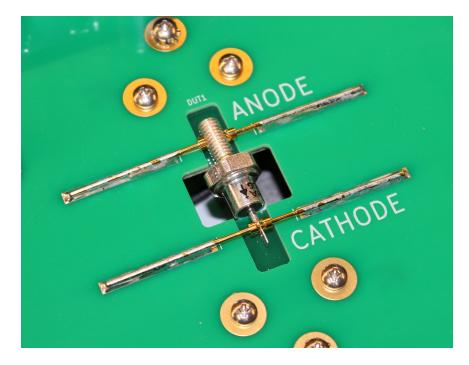
To install the diode, spread apart one pair of spring pins with your fingers or tweezers, and insert one end of the diode. Repeat on the other end.
