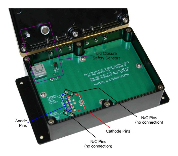
The instrument and the DUT will not be damaged if the diode is installed with the incorrect orientation (i.e., with the anode and cathode reversed). However, incorrect waveforms will be generated.
