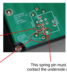
This spring pin must contact the underside of the case. It provides the cathode connection.
