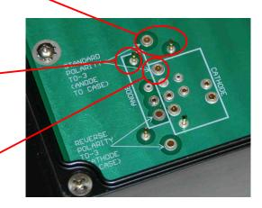
If the case is connected to the cathode, and the pin(s) are used for the anode, the arrangement shown below must be used:
