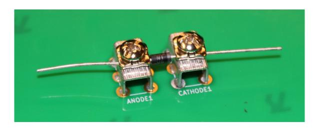
Screw and unscrew the post-screws as necessary to secure or remove the device under test.
