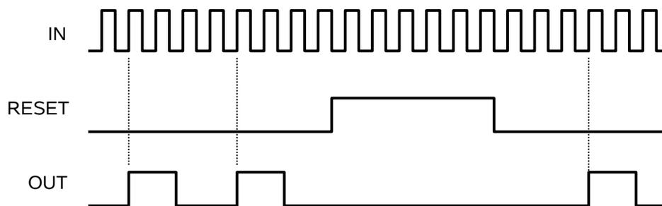
In this example,  $N=4$ . When the reset input is TTL high, the internal counter are reset to zero and are held at zero until the reset input switches to TTL low. An output pulse is generated on the fourth input pulse after the reset line returns to TTL low.
