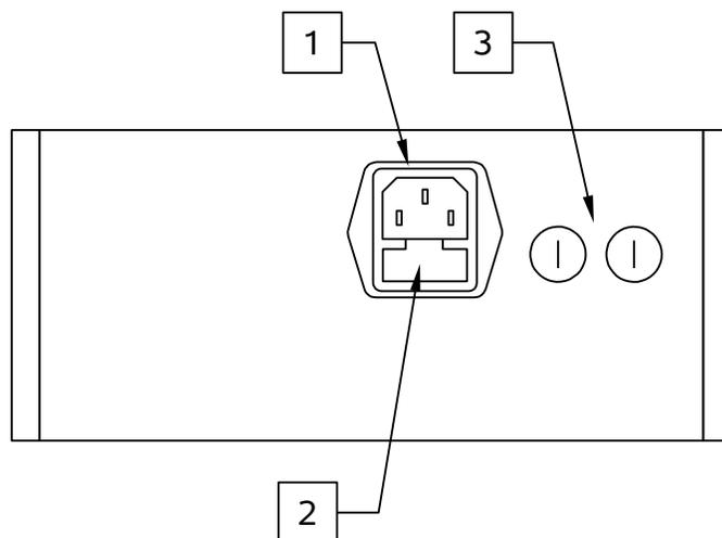
1. AC POWER INPUT. An IEC-320 C14 three-pronged recessed male socket is provided on the back panel for AC power connection to the instrument. One end of the detachable power cord that is supplied with the instrument plugs into this socket.
