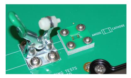
Using tweezers, position a DUT in the cavity of the raised circuit boards. The DUT will rest on four spring pins, with two contacting each DUT pad:
