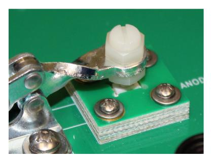
(It is possible to use a screwdriver to adjust the positioning of the nylon screw. This will vary the maximum mechanical pressure applied to the DUT.)
