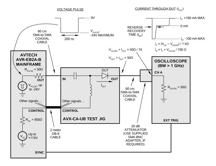
The OUT output on the test jig must be connected (using the 60 cm SMA-to-SMA cable and 20 dB attenuator supplied with the AVR-EB2A-B) to the 50 Ohm input of a highbandwidth (> 1 GHz) user-supplied oscilloscope. The voltage on the output is proportional to the current through the DUT. By observing the current waveform through the DUT, the reverse recovery time may be determined. When connected as shown above, the oscilloscope voltage waveform is related to the device current by:
