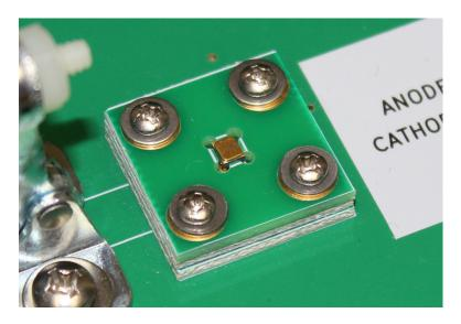
The corner notch of the DUT UB package should be in the upper right position of the photo. Refer to the label to the right of the DUT cavity.
