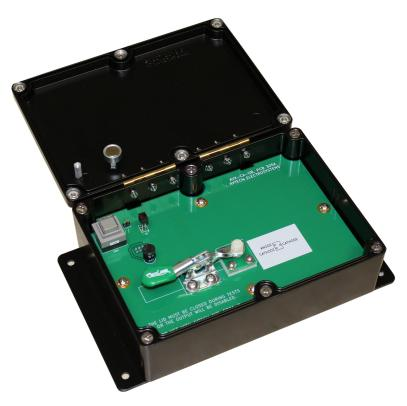
Raise the green lever on the left. This will raise the nylon screw over the DUT area on the right:
