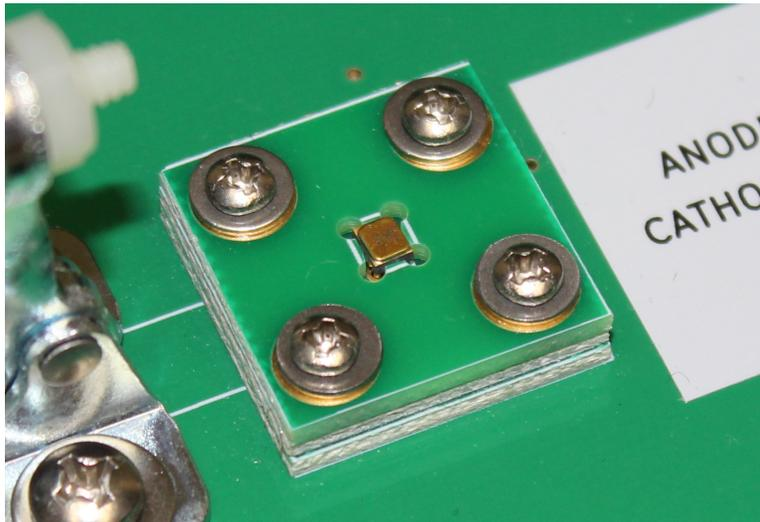
The corner notch of the DUT UB package should be in the upper right position of the photo. Refer to the label to the right of the DUT cavity.
