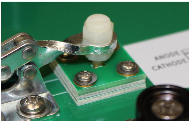
(It is possible to use a screwdriver to adjust the positioning of the nylon screw. This will vary the maximum mechanical pressure applied to the DUT.)
