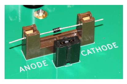
An example of a SQMELF package installed is shown below:
