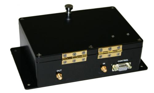
The IN, OUT, and CONTROL connectors are on the rear of the jig, below the hinges:
