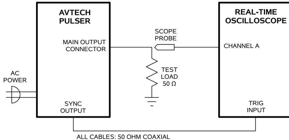
*BASIC TEST ARRANGEMENT, WITH A REAL-TIME OSCILLOSCOPE*
