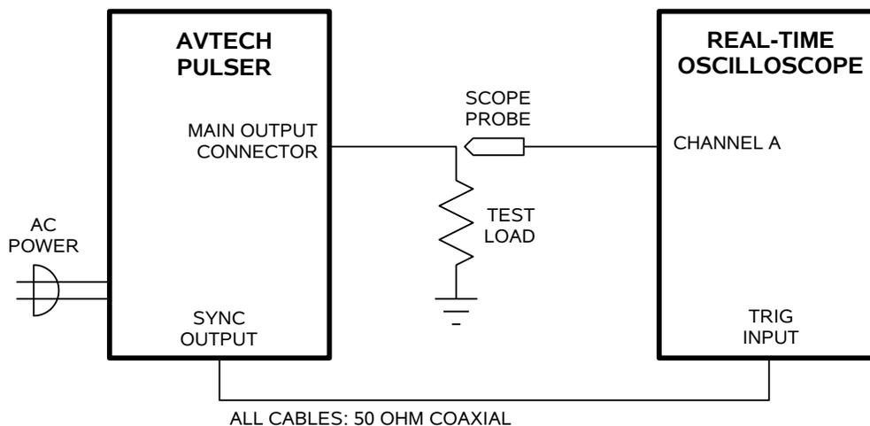
1. Connect a cable from the SYNC OUT connector to the TRIG input of an oscilloscope. Connect a 100 kΩ (or higher) load to the OUT connector and place the scope probe across this load. The load resistor must have a voltage rating of at least 400V. The power dissipated in the resistor is given by
