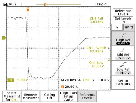
5 V/div ( = 1 A/div), 20 ns/div. 20%-80% switching time shown. S/N 11713. 5m cable used.
