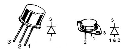
The AVX-TRR-SDA will also accept packages with reverse polarities (with the anode and cathode swapped relative to the above diagrams).
