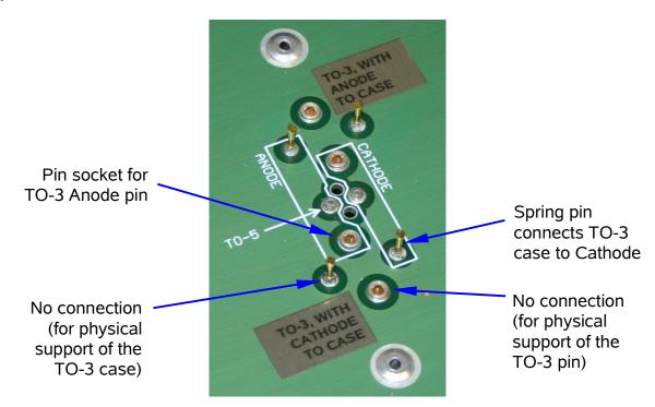
An installed case-cathode device is shown below:
