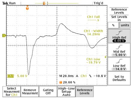
5 V/div ( = 1 A/div), 20 ns/div. 20%-80% switching time shown. S/N 11713. 5m cable used.
