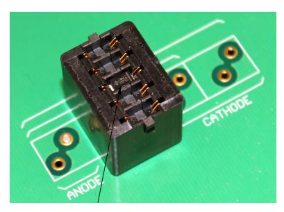
A DO214AC-packaged Device Under Test (DUT)
