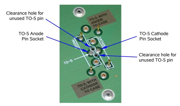
Two pin sockets are provided in the central area to accept the TO-5 package. The unconnected pin passes through one of two clearance hole in the PCB. The Anode and Cathode pin sockets are clearly marked on the PCB. The anode pin socket is on the left, and the cathode is on the right. An example installation is shown below:
