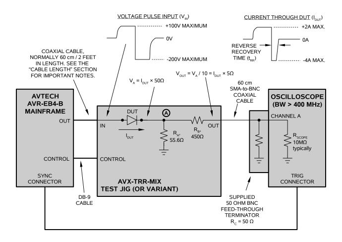
$\triangle$  A 50 Ohm resistance (R<sub>C</sub> in the diagram above) must be connected to ground on the output. This can be a discrete resistor, a feed-through terminator, or the input impedance of an oscilloscope. If a high-speed sampling oscilloscope is used, the input should be protected by adding attenuator on the input. In the diagram above, the supplied 50 Ohm feed-through terminator is used to provide the required 50 Ohm resistance.
