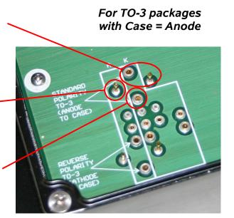
If the case is connected to the cathode, and the pin(s) are used for the anode, the arrangement shown below must be used:
