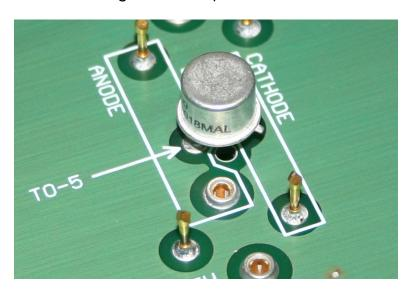
Two TO-3 configuration are possible, one with the case connected to the anode, and one with the case connected to the cathode. For the case-cathode configuration, this layout is used:
