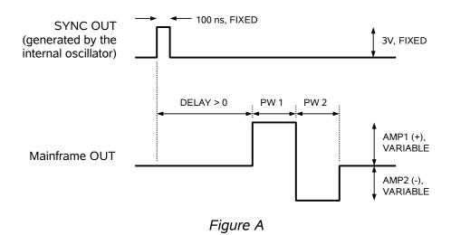
If the delay is negative, the order of the SYNC and PULSE outputs is reversed:
