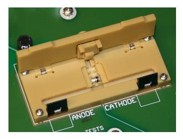
The four pockets are wired in parallel. Only one DUT may be installed at a time, or the resulting waveforms will be incorrect.
