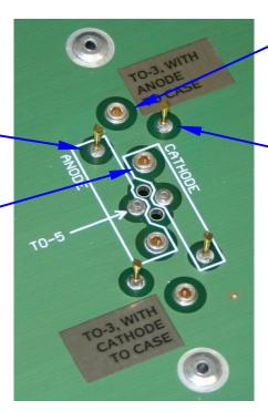
No connection (for physical support of the TO-3 pin)
