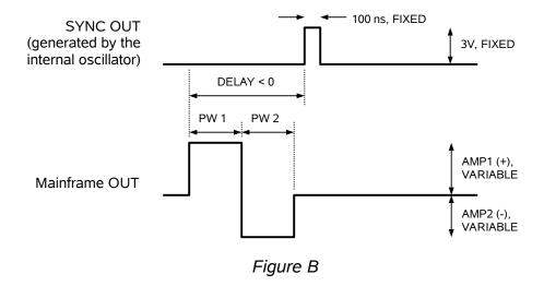
The next figure illustrates the relationship between the signal when an external TTL-level trigger is used:
