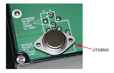
The UTG8042 has two diodes in it. For this test, only the "A" diode was tested.
