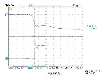
$t_r$  is measured as the 10%-90% switching time of  $V_{DS}$  (see the definitions on page 25), giving  $t_{D(ON)}$  = 1.0 ns (easily meeting the MIL-PRF-19500/564H specification of 140 ns).
