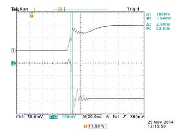
tr is measured as the 10%-90% switching time of  $V_{DS}$  (see the definitions on page 25), giving  $t_{D(ON)}$  = 2.8 ns (easily meeting the MIL-PRF-19500/557L specification of 75 ns).
