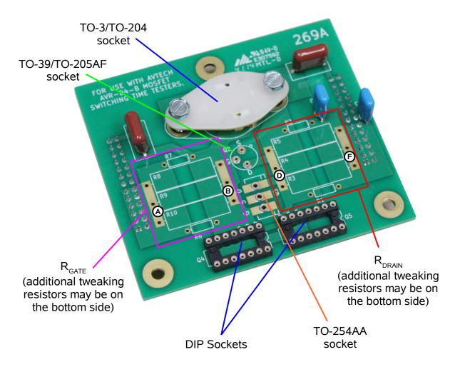
The A, B, D, and F locations correspond to the points marked in the test setup diagram on page 23. The gate, drain, and source (G, D, S) pin locations are noted on the silkscreening:
