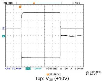
Bottom: V<sub>DS</sub> (slightly less than +30V)
