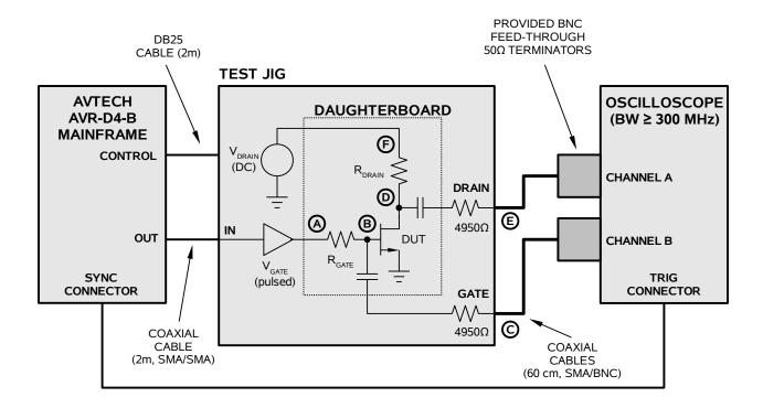
The mainframe connects to the test jig using a 2m length of SMA-to-SMA coaxial cable, and a 2m length of DB-25 cable. The cable lengths are not critical.
