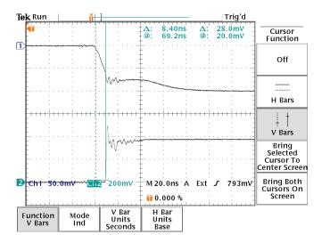
$t_{D(ON)}$  is measured from the 10% point of  $V_{GS}$  to the 10% point of  $V_{DS}$  (see the definitions on page 25), giving  $t_{D(ON)}$  = 8.4 ns (easily meeting the MIL-PRF-19500/564H specification of 60 ns).
