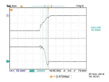
$t_{\text{D(OFF)}}$  is measured from the 10% point of  $V_{\text{GS}}$  to the 90% point of  $V_{\text{DS}}$  (see the definitions on page 25). However, in this case, the value is actually less than zero, clearly meeting the < 140 ns specification. (A greater-than-zero value would be obtained if the faster-switching voltage at the input to  $R_{\text{GATE}}$  was used as the starting reference, but Method 3472 calls for the more slowly-switching  $V_{\text{GS}}$  to be used.)
