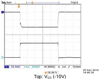
Bottom: V<sub>DS</sub> (slightly less than -40V)
