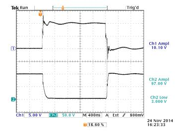
The 100:1 attenuated, AC-coupled, versions of these waveforms are provided at the test jig output connectors — points C and E in the test setup diagram on page 23:
