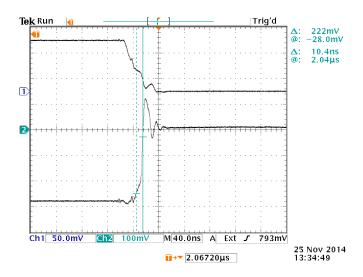
$t_{\text{D(OFF)}}$  is measured from the 10% point of  $V_{\text{GS}}$  to the 90% point of  $V_{\text{DS}}$  (see the definitions on page 25). However, in this case, the value is actually less than zero, clearly meeting the < 40 ns specification. (A greater-than-zero value would be obtained if the faster-switching voltage at the input to  $R_{\text{GATE}}$  was used as the starting reference, but Method 3472 calls for the more slowly-switching  $V_{\text{GS}}$  to be used.)
