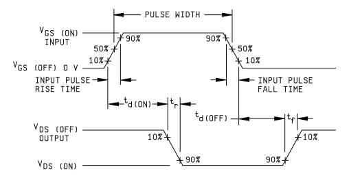
Direct access to  $V_{GS}$  (the gate waveform) and  $V_{DS}$  (the drain waveform) is not provided on the test jig output connectors. Instead, both signals pass through a capacitance in series with a  $4950\Omega$  series resistance (following the scheme used in Figure 3472-4 of MIL-STD-750-3). The  $4950\Omega$  resistance, combined with the  $50\Omega$  terminator, creates a 100:1 voltage divider.
