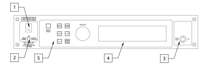
1. <u>POWER Switch</u>. This is the main power switch. When turning the instrument on, there is normally a delay of 5-10 seconds before anything is shown on the main display.
