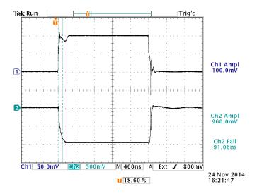
The last waveform shows a measurement of  $t_R$  of 91.06 ns. (MIL-PRF-19500/543N specifies  $t_R$  < 190 ns, so this DUT passes easily.)
