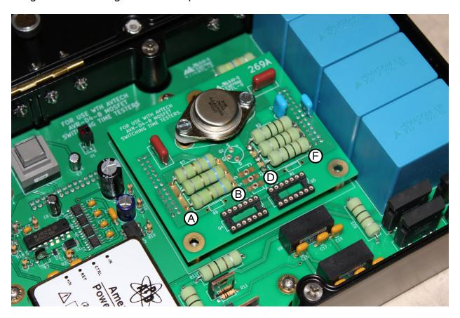
The A, B, D, and F locations correspond to the points marked in the test setup diagram on page 23. (The C and E locations are connectors on the rear panel of the jig).
