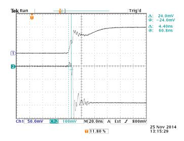
$t_{D(ON)}$  is measured from the 10% point of  $V_{GS}$  to the 10% point of  $V_{DS}$  (see the definitions on page 25), giving  $t_{D(ON)}$  = 4.4 ns (easily meeting the MIL-PRF-19500/557L specification of 30 ns).
