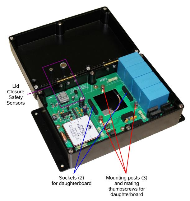
The main circuit board contains the control circuitry, gate driver circuitry, and the high-voltage bipolar power supply for the drain bias.
