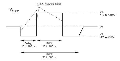
In the waveform shown above, a wide negative pulse (with pulse width PW2 and amplitude -V2) is interrupted by a shorter positive pulse (PW1, +V1). The three highlighted transition have switching times of 20 ns or less. (The final transition to ground is slower).
