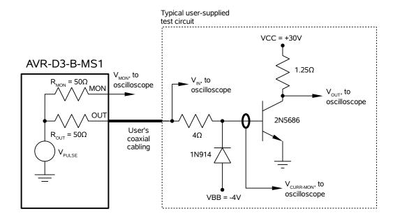
A 50 Ohm output impedance exists between the internal pulse generator circuit and the output connector on the front panel of the instrument.
