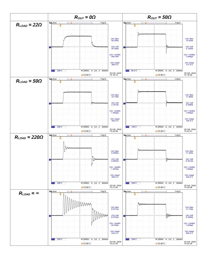
It should be observed that maximum voltages are obtained when  $R_{OUT} = 0\Omega$ , but transmission line reflections are minimized with  $R_{OUT} = 50\Omega$ . Also, regardless of the value of  $R_{OUT}$ , reflections and ringing are minimized when  $R_{LOAD} = 50\Omega$ .
