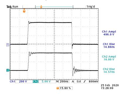
Top: +500V pulse, internally (before ROUT) Bottom: resulting +10A current, measured with a CT2 current probe (1V/A).
