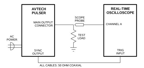
1. Connect a cable from the SYNC OUT connector to the TRIG input of an oscilloscope. Connect a 50 $\Omega$  (or higher) load to the OUT connector and place the scope probe across this load. The load resistor and the scope probe <u>must</u> have a voltage rating of at least 1000V. The power dissipated in the resistor is given by
