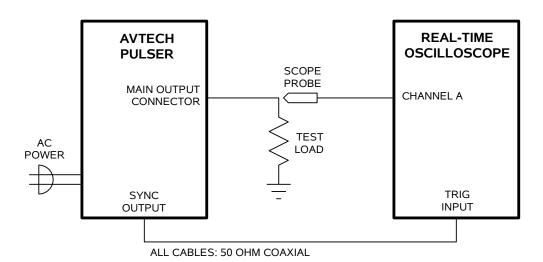
1. Connect a cable from the SYNC OUT connector to the TRIG input of an oscilloscope. Connect a  $50\Omega$  (or higher) load to the OUT connector and place the scope probe across this load. The load resistor <u>must</u> have a voltage rating of at least 500V. The power dissipated in the resistor is given by
