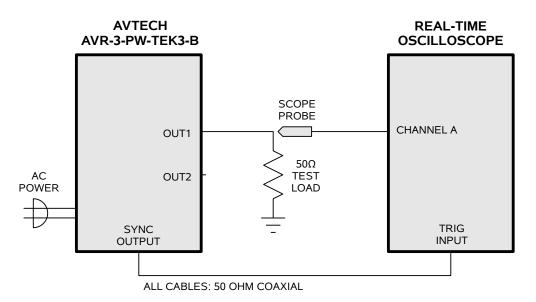
A high-quality low-inductance 50 Ohm load is required for the above test arrangement. The worst case power dissipation in the load resistor is 3.1 Watts.
