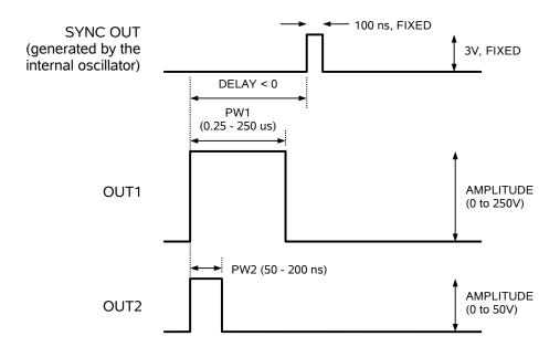
The next figure illustrates the relationship between the signals when an external TTLlevel trigger is used:
