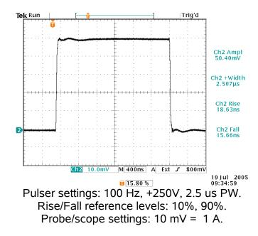
The probe is slower than the input pulse, so the measured rise time is slower. The probe also introduces a small amount of ringing.
