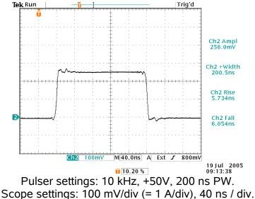
Larger values of attenuation (> 6 dB) will reduce the reflections (and the pulse amplitude) further.
