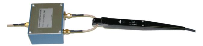
The OUT1 and OUT2 connectors are different. OUT1 has a BNC connector, and OUT2 has an SMA connector. The output modules have matching connectors, to make it obvious which output module is to be used with which output connector.
