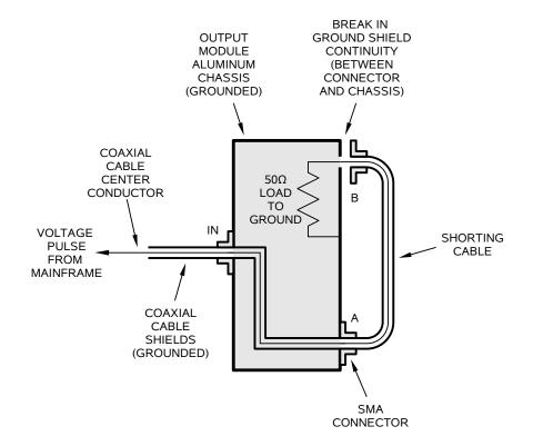
The connectivity of the ground shield of the shorting cable is deliberately broken so that current can not flow in the shield - if the cable shield was active, it would prevent the current probe from sensing the current on the center conductor!
