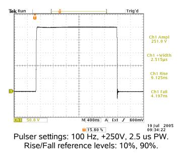
When OUT1 is connected to the AVX-TEK3-TM1 (using the arrangement shown in the "BASIC TEST ARRANGEMENT, WITH OUTPUT MODULES" section) and a Tektronix A6303 probe system, waveforms similar to the one shown below will be obtained:
