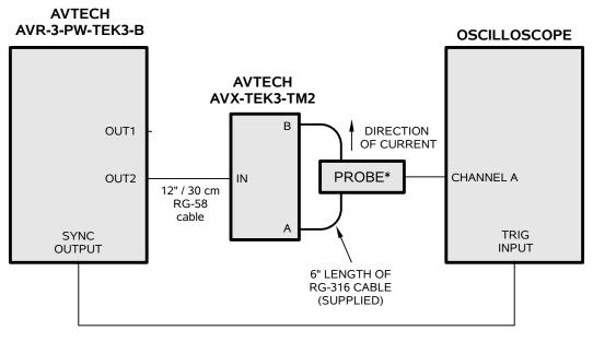
\* Depending on the exact current probe model, a probe amplifier may be needed between the probe and the oscilloscope.
