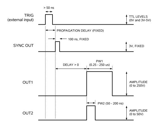
The delay, pulse width, and frequency (when in the internal mode), of the OUT pulse can be varied with front panel controls or via the GPIB or RS-232 computer interfaces.
