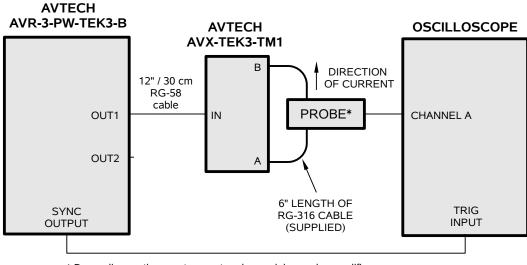
\* Depending on the exact current probe model, a probe amplifier may be needed between the probe and the oscilloscope. The current probe under test is clamped to the 6" / 15 cm length of RG-316 cable across the "A" and "B" terminals of the output module. Physically, this arrangement is shown below (with a Tektronix A6303 probe):
