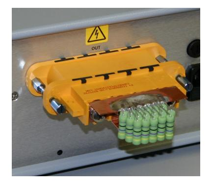
In both cases, the OUTPUT signal is provided on the NARROW copper strip, and the GROUND is provided on the WIDE copper strip. This is shown schematically below:
