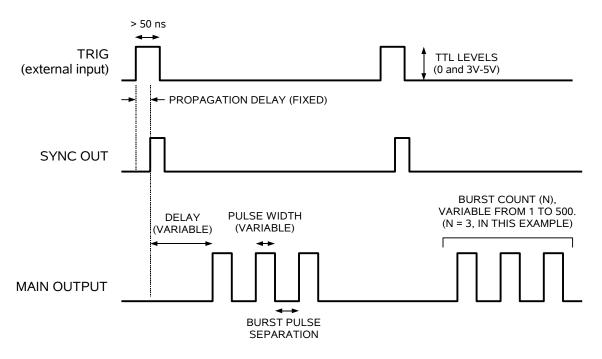
The burst mode may also be used with the front-panel "Single Pulse" pushbutton as a trigger source. (Pressing the pushbutton will actually generate a single burst, rather than a single pulse, in this mode.) Computer commands can also trigger a burst.
