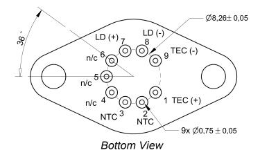
The LD(-) pin (the cathode) is grounded. The positive signal is applied to the LD(+) pin (the anode).
