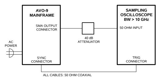
Since most sampling oscilloscopes have limited input amplitude ranges, attenuators are required. Select appropriate attenuators for your oscilloscope.
