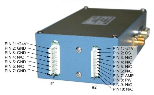
Connectors #1 and #2 are shown above. These supply the DC power and the amplitude and pulse width signals to the module, as well as any required DC offset for the output.
