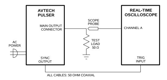
BASIC TEST ARRANGEMENT, WITH A REAL-TIME OSCILLOSCOPE
