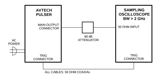
BASIC TEST ARRANGEMENT, WITH A SAMPLING OSCILLOSCOPE
