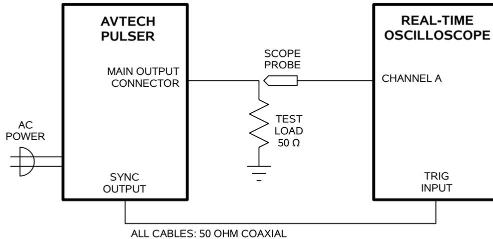
*BASIC TEST ARRANGEMENT, WITH A REAL-TIME OSCILLOSCOPE*
