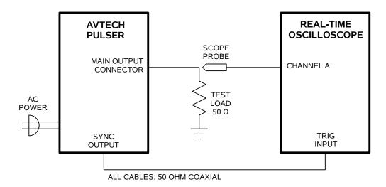
BASIC TEST ARRANGEMENT, WITH A REAL-TIME OSCILLOSCOPE
