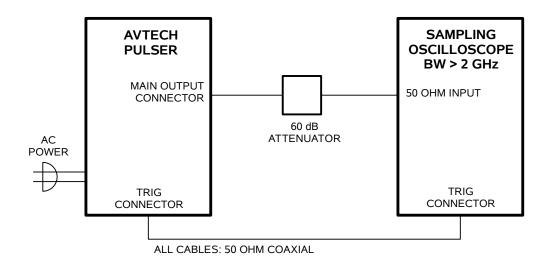
BASIC TEST ARRANGEMENT, WITH A SAMPLING OSCILLOSCOPE
