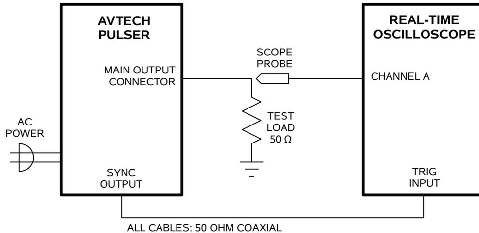
*BASIC TEST ARRANGEMENT, WITH A REAL-TIME OSCILLOSCOPE*
