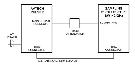
BASIC TEST ARRANGEMENT, WITH A SAMPLING OSCILLOSCOPE
