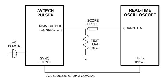
BASIC TEST ARRANGEMENT, WITH A REAL-TIME OSCILLOSCOPE
