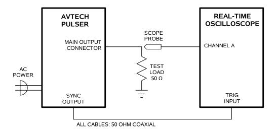
BASIC TEST ARRANGEMENT, WITH A REAL-TIME OSCILLOSCOPE
