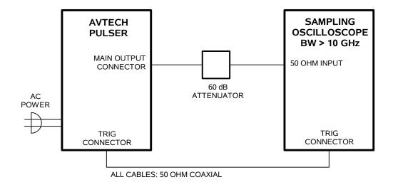
BASIC TEST ARRANGEMENT, WITH A SAMPLING OSCILLOSCOPE
