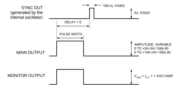
Basic Output Pulses for Delay < 0
