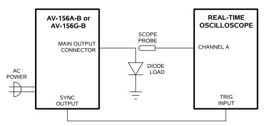
Reversing this connection may cause the diode to breakdown, possibly damaging it.
