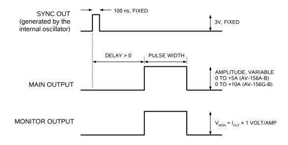
Basic Output Pulses for Delay > 0
