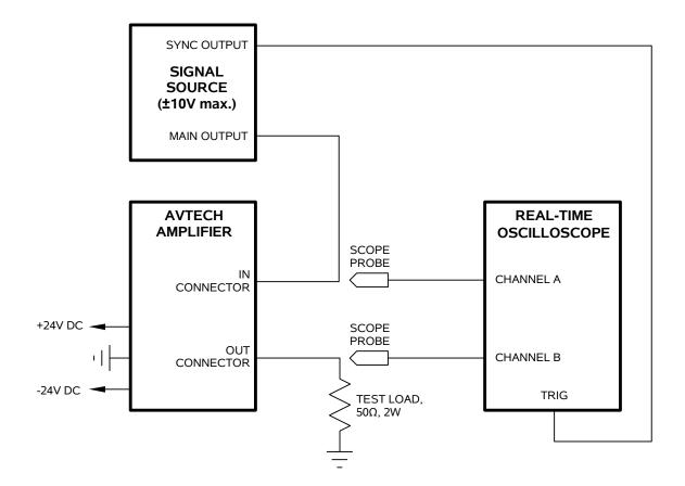
The recommended test set-up is shown above. The Avtech AV-1000-C pulse generator is a suitable signal source.
