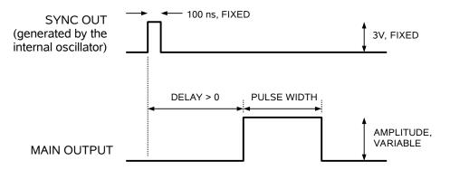
Basic Output Pulses for Delay > 0
