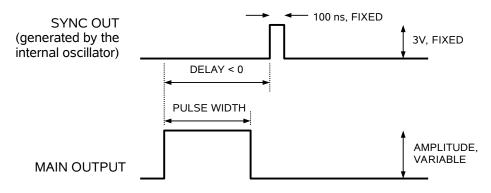
Basic Output Pulses for Delay < 0
