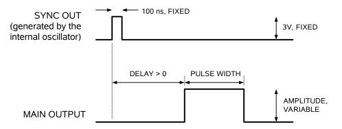
Basic Output Pulses for Delay > 0
