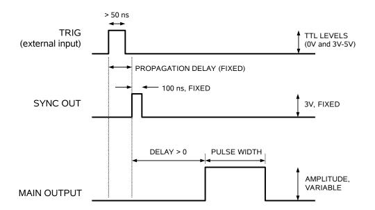
As before, if the delay is negative, the order of the SYNC and OUT pulses is reversed.
