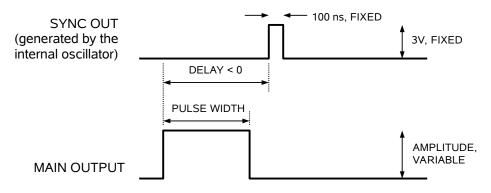
Basic Output Pulses for Delay < 0
