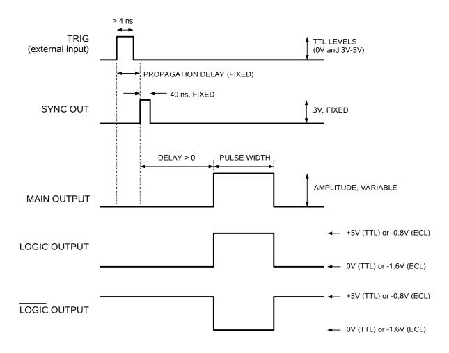
As before, if the delay is negative, the order of the SYNC and OUT pulses is reversed.
