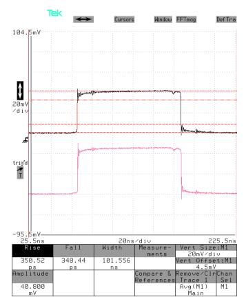
Top: Voltage measured across the resistor in response to a +4.8V pulse applied from an Avtech AV-1030-C pulse generator. It should be approximately  $(+4.8V / 54.6\Omega) \times 4.6\Omega = 404$  mV, which agrees with the observed waveform. 200 mV/div (= 20 mV/div × 20 dB), 20 ns/div.
