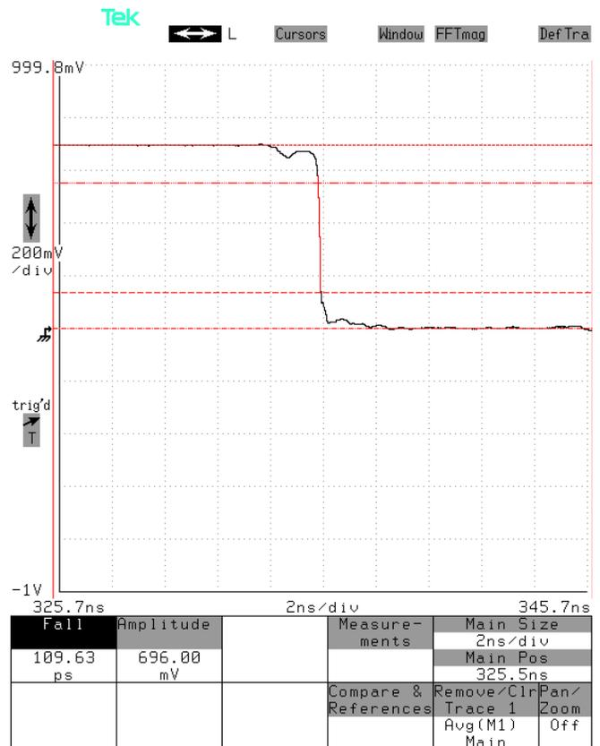
The output rise time should be less than  $\sqrt{((99.38\text{ps})^2 + (60\text{ps})^2)} = 116.1 \text{ ps}$ . The measured rise time does satisfy this limit.
