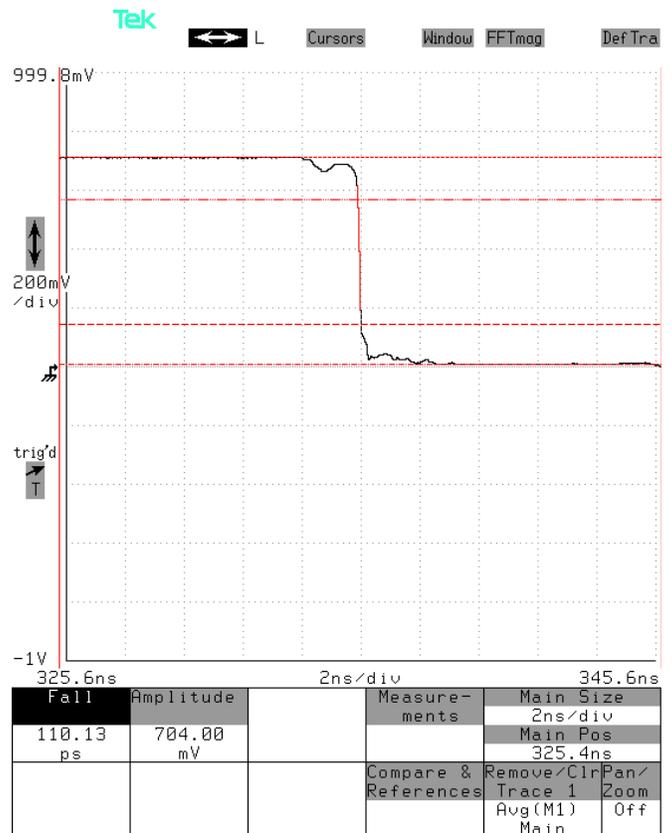
The output rise time should be less than  $\sqrt{((100.61ps)^2 + (60ps)^2)} = 117.1 ps$ . The measured rise time does satisfy this limit.
