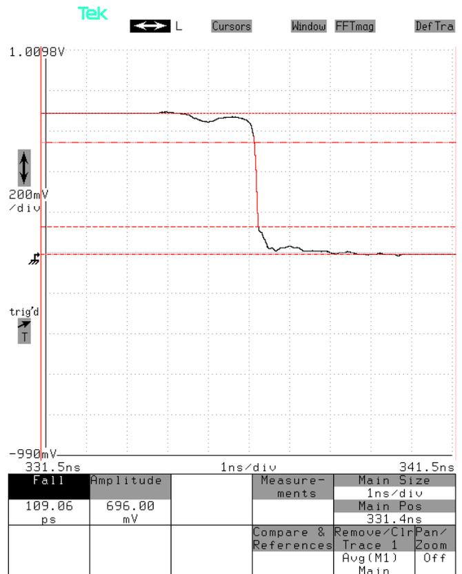
The output rise time should be less than  $\sqrt{(99.59ps^2 + 60ps^2)} = 116.3$  ps. The measured rise time does satisfy this limit.
