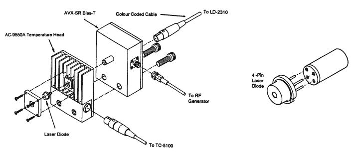
FIGURE 4 - AVX-SR ASSEMBLED WITH AC-9550A TEMPERATURE HEAD
