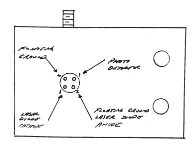
AUX - SRB PIN CONNECTONS (TYDE-1) CLASER DIODE PIN SECIET)
