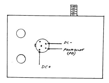
AUX-SRB PIN CONNECTIONS (TIPE 2) (De BIAS + PHOTO DIOPE)
