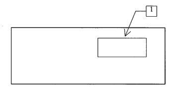
1. <u>AC POWER INPUT</u>. A three-pronged recessed male connector is provided on the back panel for AC power connection to the instrument. Also contained in this assembly is a 0.5A slow blow fuse and a removable card that can be removed and repositioned to switch between 120V AC in and 240V AC in.
