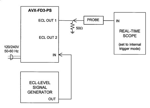
Test Arrangement for Real-Time Scopes
