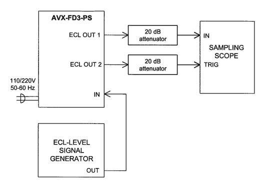
Test Arrangement for Sampling Scopes
