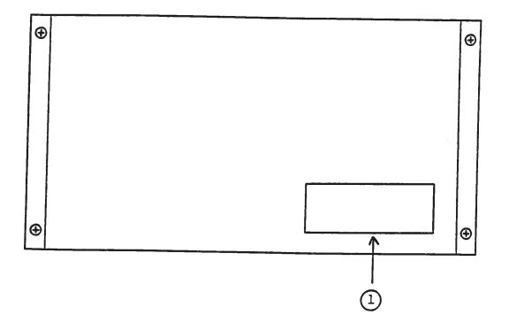
(1) <u>FUSED CONNECTOR, VOLTAGE SELECTOR</u>. The detachable power cord is connected at this point. In addition, the removable cord is adjusted to select the desired input operating voltage. The unit also contains the main power fuse. (0.5 A SB).
