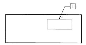
1. <u>AC POWER INPUT</u>. A three-pronged recessed male connector is provided on the back panel for AC power connection to the instrument. Also contained in this assembly is a 1/2A slow blow fuse and a removable card that can be removed and repositioned to switch between 120V AC in and 240V AC in.
