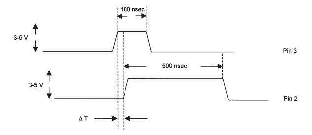
As the PW pot is varied over its full range  $\Delta T$  should vary from about 0 to approximately 100 nsec. If the waveforms at pins 2 and 3 do not resemble the above, then the -T module is defective and should be replaced. If the waveforms do resemble the above then the -PG module is at fault and should be replaced.
