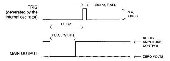
When triggered externally, the TRIG connector acts as an input. This illustrated below:
