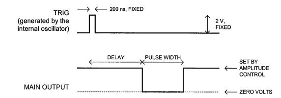
When the ADVANCE/DELAY switch is set to "DELAY", the TRIG output occurs after the main output. This illustrated below:
